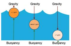
density will float somewhere in the middle of the fluid, this is called neutral buoyancy (middle of diagram).
