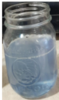
This is Thunder Bay tap water and cabbage juice. It is visibly more blue, and sits at about an 8 on the pH scale. This means that the water is slightly alkaline. This makes sense, because the city added sodium hydroxide to their water to balance out the lead in it. Sodium hydroxide sits at about 13 on the pH scale.
